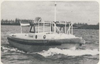
The picture on top of this page, shows the Spurt 25 put into practice under classified specification, for tropical conditions, which proves again the quality of the fibreglass hull, sandwich deck and design: **the Spurt 25 as a mooring launch.** The heavy mooring ropes demand a lot of power: 100 h.p. marine diesel engines have been built in and a special cleat for automatic handling of the heaviest ropes has been installed on the sandwich deck.
